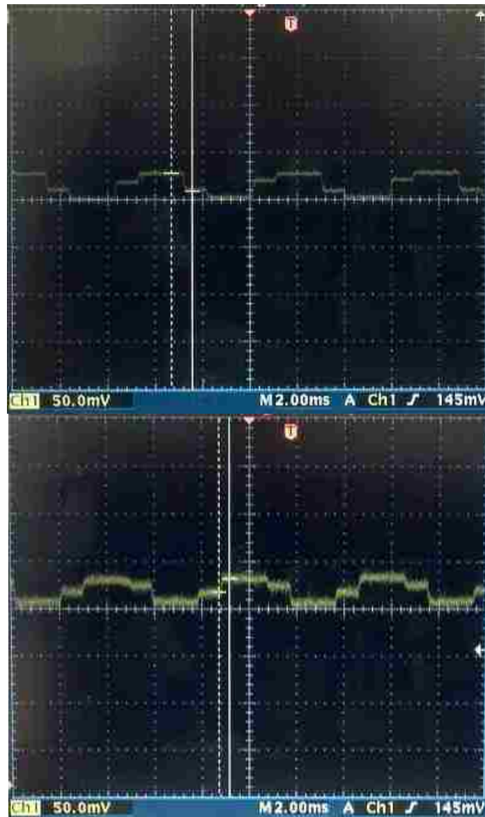
Figure 2.11 – Measured skin displacement for LRA devices. Top: Block design.
