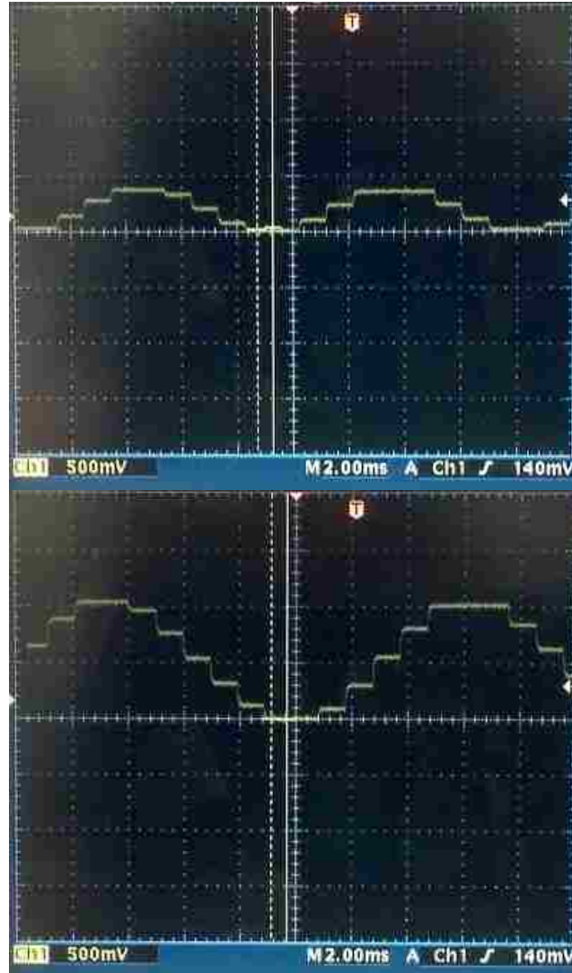
Figure 2.12 – Measured skin displacement for ERM devices. Top: Block design. Bottom: Suspension design. *Note the different scales between Figure 2.11 and Figure 2.12.
