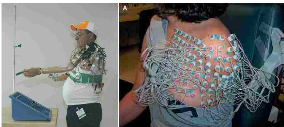
Figure 5.2 – Left: Subject performing the Clothespin Relocation task [128]. Right: subject fitted with an array of EMG sensors to map muscle activity following TMR [129].
