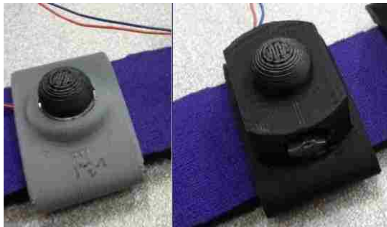
Figure 2.4. – Original block holders mounted on a purple elastic band. (Left) Block LRA holder, (Right) Block ERM holder.
